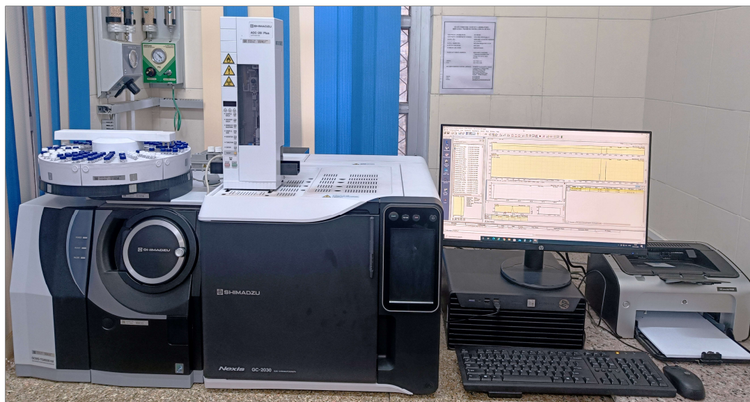
A view of Gas Chromatograph-Mass Spectrometer (Triple Quadrupole)
